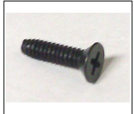
US800735 - END CAP SCREW FASTNER 10-24 x 3/4" FH PH THREAD RING MS (BLACK OXIDE, BOTTOM LOAD)
