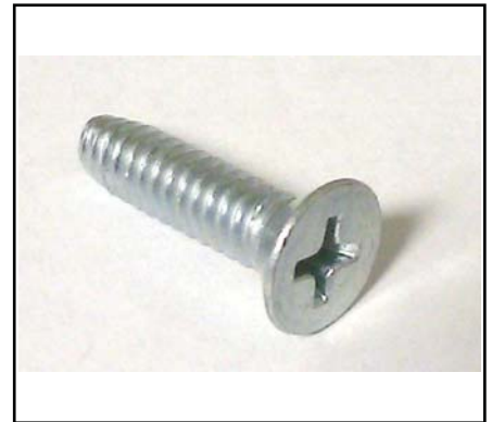
US800706 - END CAP SCREW FASTNER 10-24 x 3/4" LG PH FL HD THREAD ROLLING ZP MS (ZINC OXIDE, BOTTOM LOAD)
